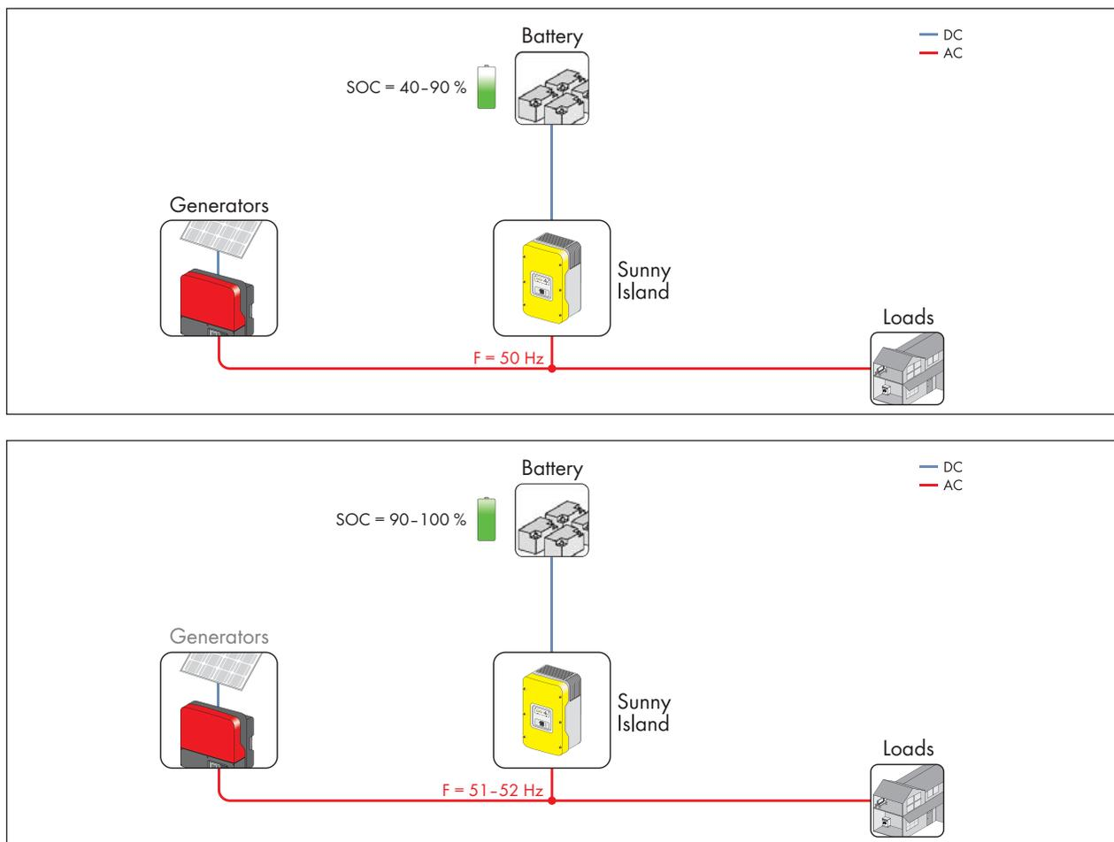
Fig. 1: At a charge of lower than 90 percent, the battery absorbs power surpluses at any time. When the battery is fully charged and power surpluses exist, the Sunny Island increases the AC frequency and the generators accordingly reduce their power output.
