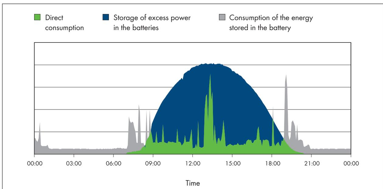
Fig. 5: Example of a daily overview of the three possible energy states of an off-grid system
