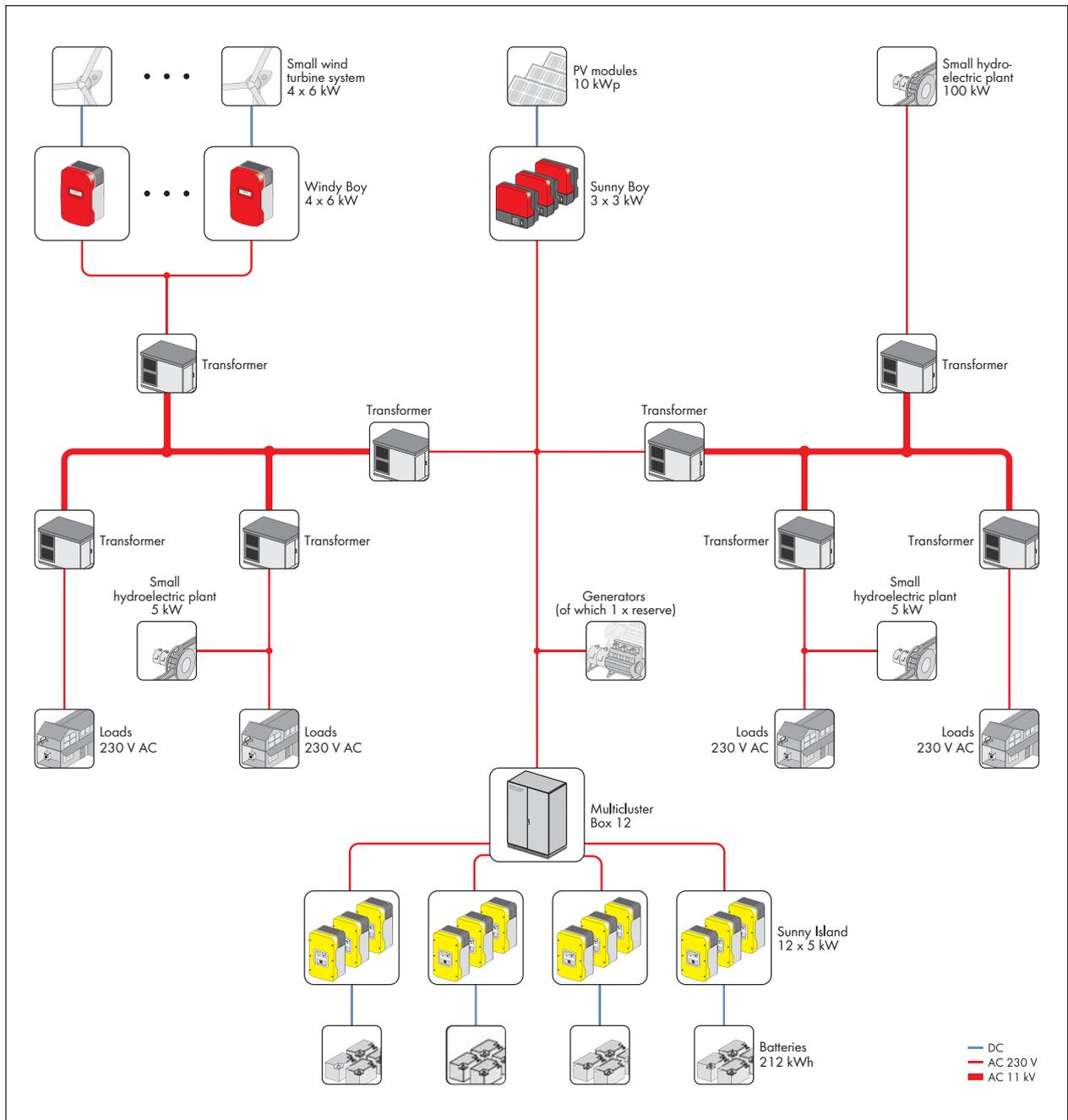
Fig. 4: Schematic of Eigg Island power supply structure
