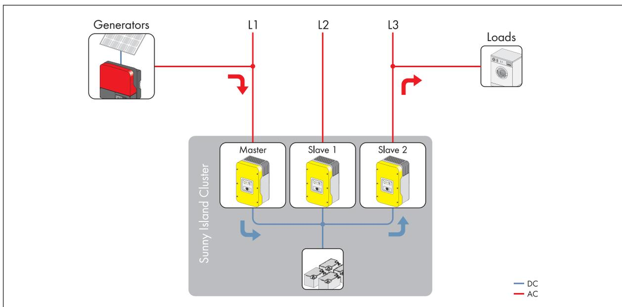
Fig. 2: Asymmetric load on the three-phase grid is no problem
