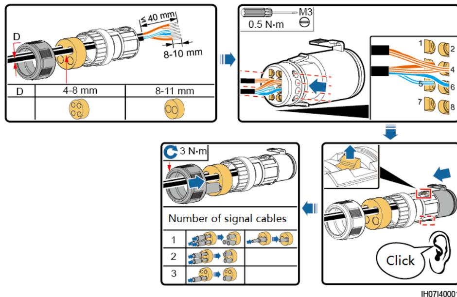
**Figure 5-26** Assembling a signal connector (SUN2000 cascading)
