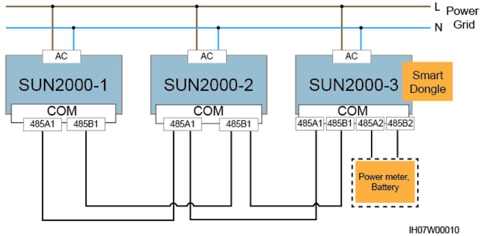
**Figure 5-22** Connecting cables to the power meter (in-phase grid connection)
