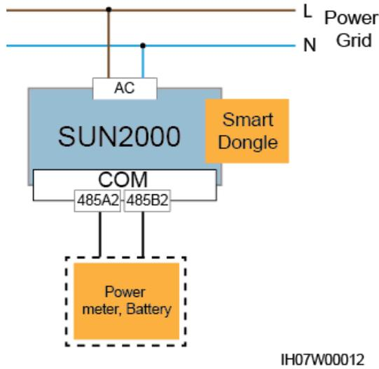
**Figure 5-20** Connecting cables to the power meter (single SUN2000)
