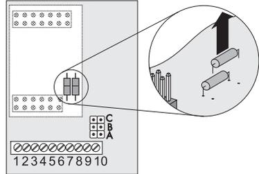
3. Plug the communication interface (A) to the left of the interface port. The 2 pins on the right of the short pin row below stay free.
