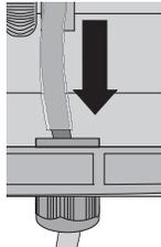
5. For simplification the two cables can be bound together with a cable tie.
