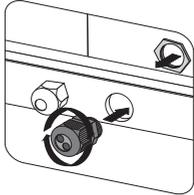
4. Unscrew the nut of the cable gland and push out the seal insert.
