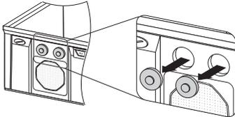
3. Place the cable gland with single seal insert into the prepared enclosure opening of the inverter and fasten it with a nut from inside the enclosure.
