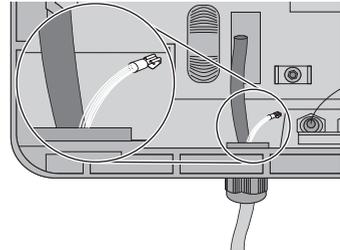
3. Tighten the nut of the cable gland to secure the cable.
