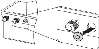
3. Insert the cable gland with the double seal insert into the enclosure opening of the inverter and fasten it from inside with a nut.
