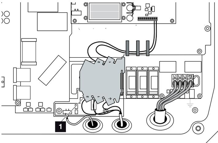
Fig. 65: RS485 overvoltage protection in the inverter
