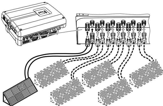
Fig. 32: Overview of DC connections
