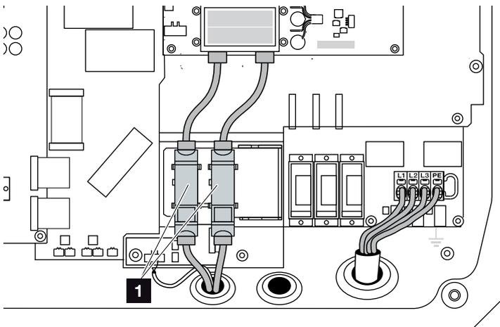
Fig. 29: LAN overvoltage protection
