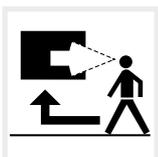
Inverters must be easily accessible and the display clearly visible.
