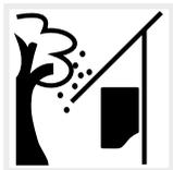
Protect inverter from falling parts which could enter the inverter's ventilation openings.
