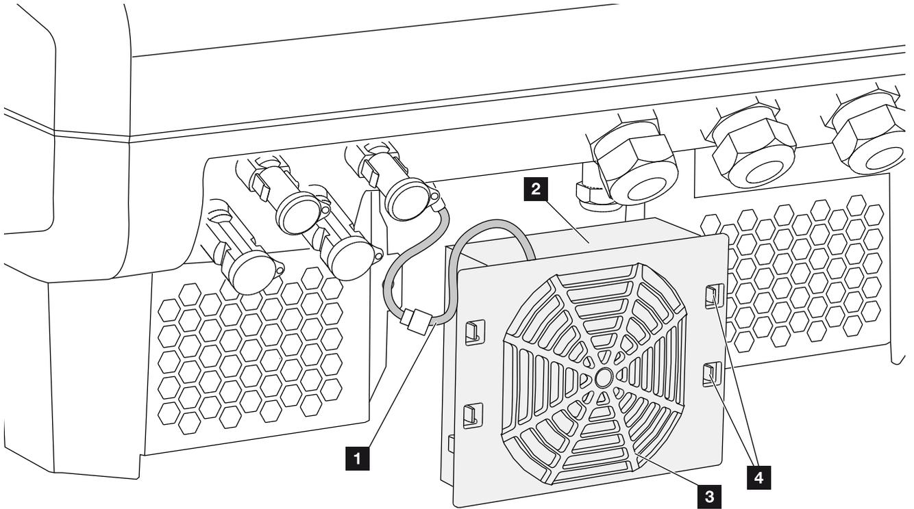
Fig. 56: Fan disassembly overview
