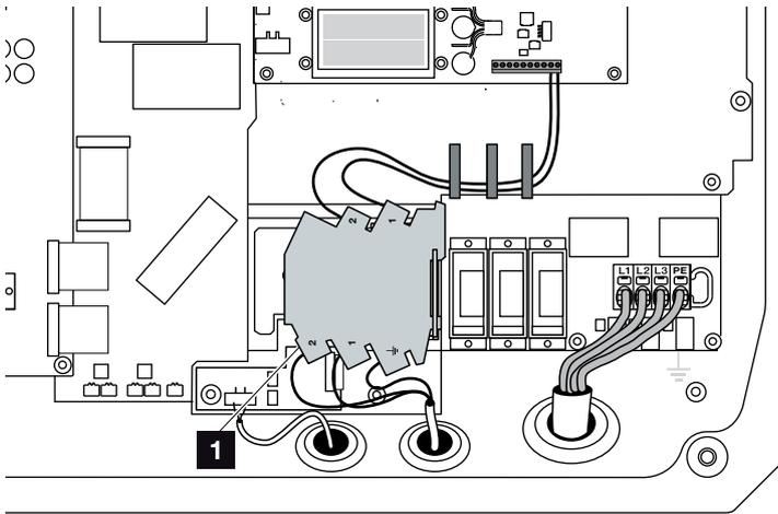
Fig. 30: RS485 overvoltage protection in the inverter
