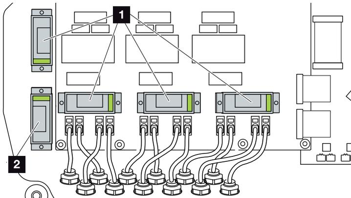
Fig. 62: Installation positions for DC overvoltage protection
