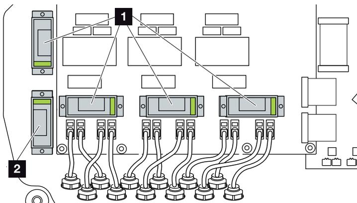
Fig. 26: Installation positions for DC overvoltage protection
