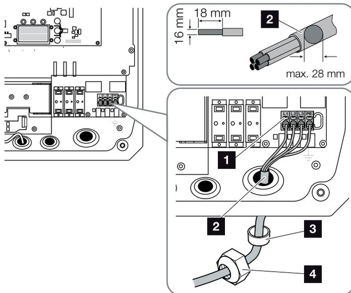
Fig. 21: Connect mains cable to the inverter
