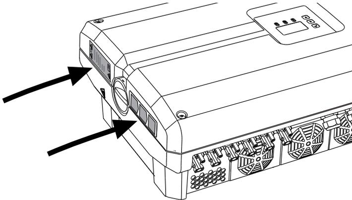
Fig. 7: Labels on the inverter – Figure example
