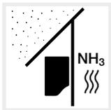
Protect the inverter against dust, contamination and ammonia gases. Rooms and areas containing livestock are not permitted as installation sites.
