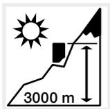
Inverter may only be installed up to an altitude of 3000 m. (Derating as of 2000 m)
