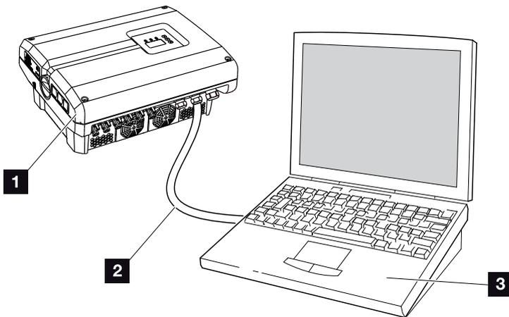
Fig. 49: Connect the inverter and computer directly
