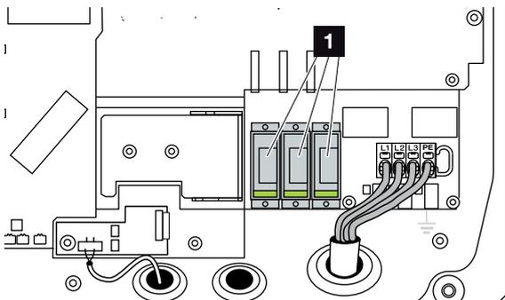
Fig. 63: Installation positions for AC overvoltage protection
