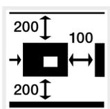
Maintain minimum distances to other inverters and the necessary clearance.
