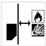
A sufficient safety distance from flammable materials and potentially explosive areas in the vicinity must be ensured.
