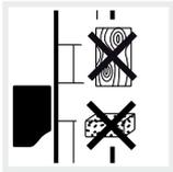
Mount inverter on a stable installation surface that can safely bear the weight. Plasterboard walls and wood planking are not permitted.
