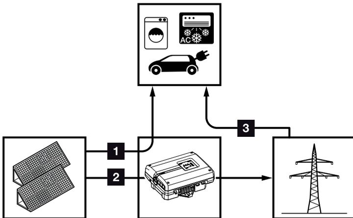
Fig. 46: Control and distribution of the energy flows
