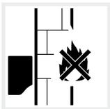
Mount inverter on a non-flammable installation surface.
