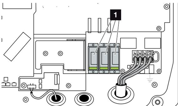
Fig. 27: Installation positions for AC overvoltage protection
