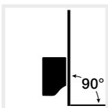
Mount inverters on vertical installation surfaces. For this purpose, use the wall mount provided.
