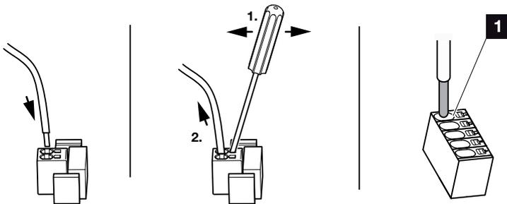
Fig. 22: Spring-loaded terminal strip
