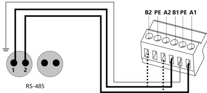
3. The inverters are connected to the ShineMaster via RS485 serial connection. Using the RS485 wired communication connection, the ShineMaster can monitor up to 32 inverters stably.
