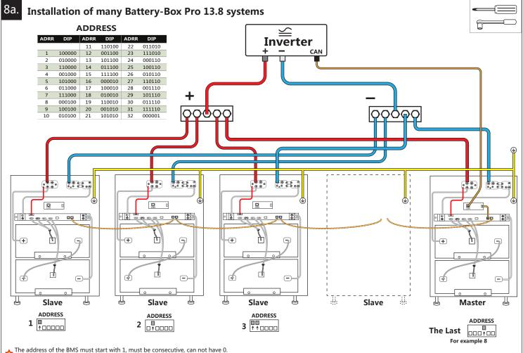
The address of the BMS must start with 1, must be consecutive, can not have 0. Only the BMU with the last address is connected to the inverter.
