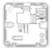
Connect the live and neutral AC mains (marked AC IN 110-240v). This feed should come from the fused spur.
