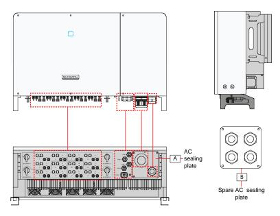
Fig.2. Wiring Terminals (Take SG250HX as an example)
