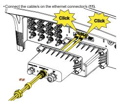
•Install the signals connection box (08) by screwing the 4 locking screws present on it (see paragraph "3.5.2 Tightening torques").
