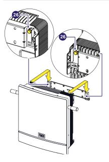
• Remove the handles (25) or eyebolts and tighten the supplied two side bracket screws (18) (see paragraph "3.5.2 Tightening torques") to avoid the tilting of the bottom part of the inverter.
