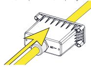
•If the AC cable have a diameter between 20...26 mm should be installed the supplied reducing seal.
