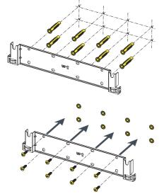
· Attach the bracket (05) to the support.
