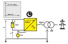
Array terminal voltages with respect to ground during night-time PID recovery operation (inverter is off-line).
