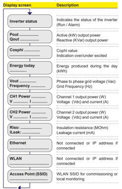
NOTE – The visualization of the parameters change every 15sec or every time the button ♥ is pressed.
