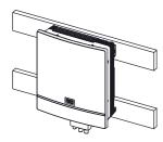
•The vertical installation of two inverters positioned back to back is also permitted on a structure which must be composed of a support for the attachment of the brackets and one for the support of the rear pins.
