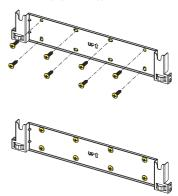
• In case of use of "frame fixing brackets" it will be possible to fix the bracket to the frame structure without drill any holes.
