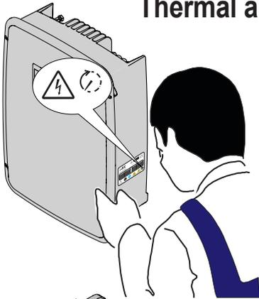
**WARNING:** the removal of guards or covers is only permitted after the voltage has been removed and time period indicated on the label has passed. This is to let the components cool down and allow the internal capacitors to discharge. Refer to “Inverter switch-off” chapter on this manual to know all the necessary step to safely operate on the inverter.
