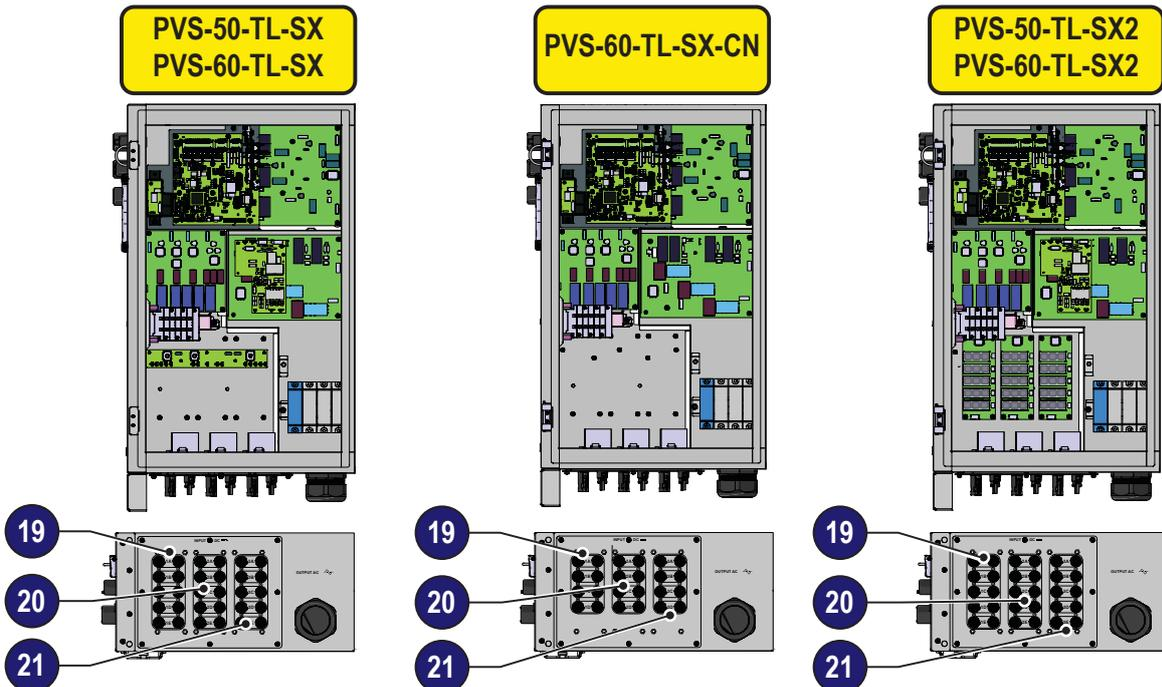
Refer to the document “String inverter – Product Manual appendix” available at [www.fimer.com](http://www.fimer.com) to know the brand and the model of the quick fit connector. Depending on the model of the connector of the own inverter, it is necessary to use the same model and the respective counterpart (check the compliant counterpart on the website of the manufacturer or in FIMER)
