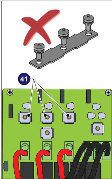
In the inverter -SX and -SX2 versions, the independent configuration of the input channels (MPPT) is set at the factory. This means that the parallel bar (supplied) must not be installed on the parallel MPPT connection points 41, and that the software setting “Independent channel mode” should be performed on the inverter; this setting can be done by different way:
