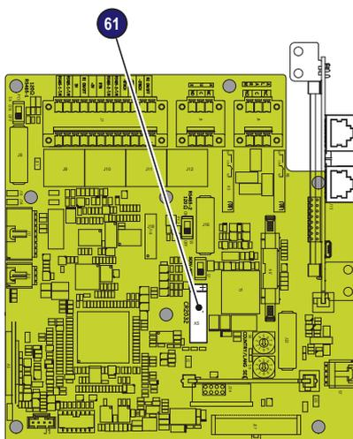
Replacing the buffer battery (61) is carried out on the wiring box and may be necessary in the following circumstances:
