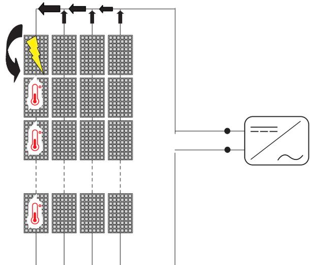
In these versions, you must directly connect the individual strings coming into the inverter (do not make field switchboards for parallel strings). This is because the positive side (+) <sup>35</sup> and negative side (-) <sup>34</sup> string fuses, situated on each input, are not rated to take strings in parallel (array). This operation can cause damage to the fuse and consequently malfunctioning of the inverter.
