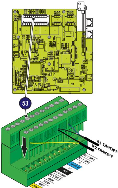
The connection and disconnection of the inverter to and from the grid can be controlled through an external control. The function must be enabled in the relevant menu through the Aurora Manager Tools software. If the remote control function is disabled, the switching on of the inverter is dictated by the presence of the normal parameters which allow the inverter to connect to the grid.
