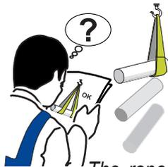
*The ropes and equipment used for lifting must be suitable for bearing the weight of the equipment.*
