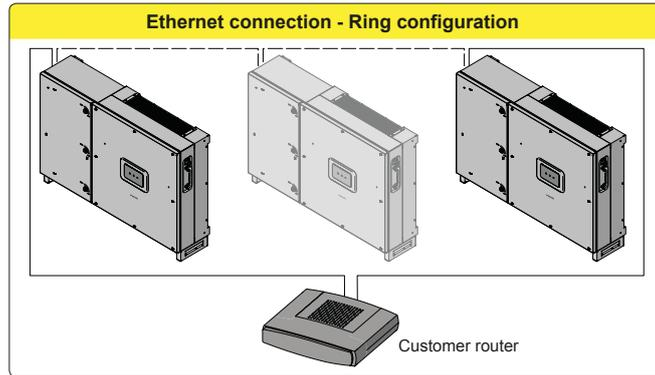
The ring configuration is the preferable way to connect the units in order to allow reaching inverters in case of single inverter fault.
