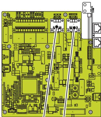
The inverter is equipped with 2 multifunction relays with configurable activation. It can be connected with normally open contact (being connected between the NO terminal and the common contact C) and with normally closed contact (being connected between the NC terminal and the common contact C).
