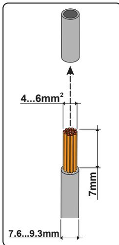
Installation of Amphenol H4 connectors requires crimping to be carried out with suitable equipment.
