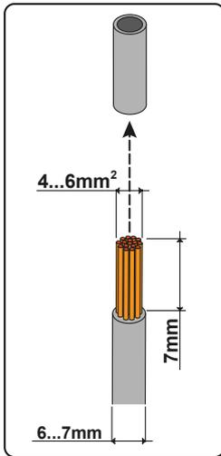
Installation of Weidmüller WM4 connectors requires crimping to be carried out with suitable equipment.
