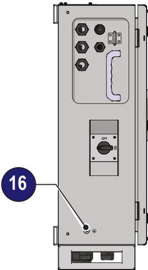
As alternative is possible to connect the earth cable to the protective earth terminal (external) 16 positioned on the left side of the mechanics. As per the protective earth terminal (internal) 37 following to the sequence illustrated in the below figure and tightening it to a torque of 11Nm. A ring cable lug, suitable for a M6 size threaded insert, must be installed on the cable.
