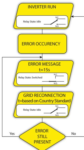
Selectable alarms for which the relay is activated
