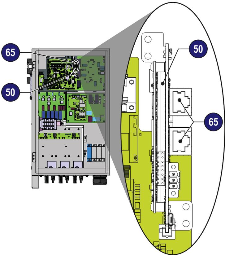
Connection of ethernet cable is made trough the two RJ45 connectors 65.
