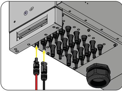
For the string connections on the -SX /-SX2 versions, it is necessary to use the quick fit connectors (usually Weidmüller PV-Stick or WM4, Multi-Contact MC4 and Amphenol H4) located on the bottom of the mechanic. The input connectors are divided into 3 groups (one group for each input channel) consisting of 5 pairs (4 pairs for the PVS-60-TL-SX-CN model) of quick fit connectors.
