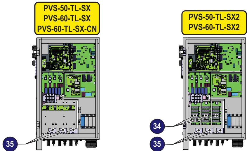
A “return current” can be generated in the event of a fault and relevant short-circuit at the ends of one or more PV modules of the system; this condition can cause all the current supplied by the strings not involved in the fault, but connected to the same input channel, to pass through the faulty string.
