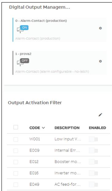
This section of the menu allows you to set the activation status of a relay (available either as contact normally open – N.O. - and as a normally closed contact -N.C.) and to configure customised alarm conditions.
