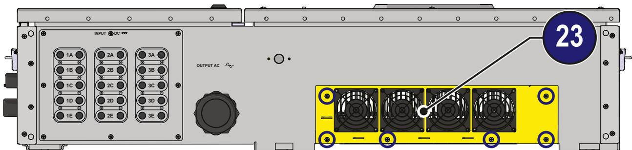
3. Pull out the cooling section
