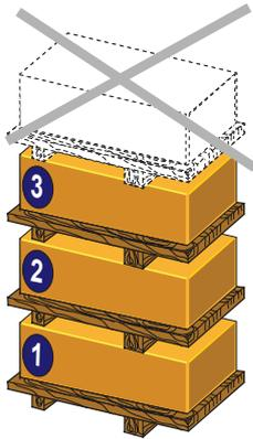
If the package is stored correctly, it can withstand a maximum load of 3 stacked devices (divided into 3 pallets).
