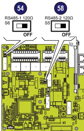
When an RS-485 connection is being used, if one or more inverters are added to the system at a later time, it is necessary to remember to reset to OFF the switch on the termination resistance being used (1) or (2) on the inverter which previously was the last in the system.
