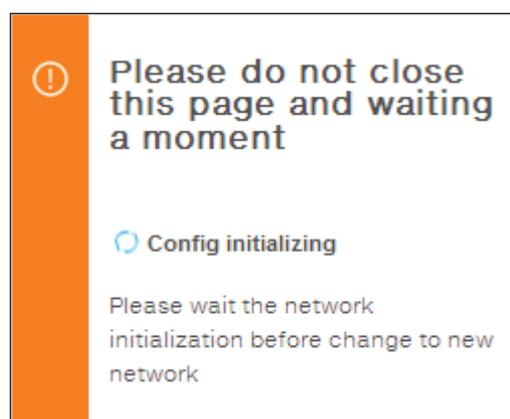
Once the inverter is associated with a wireless network, the user must switch the tablet/smartphone/PC to the same wireless network which the inverter is connected.
