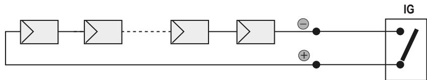
Once the short-circuit has been made, measure the isolation resistance (Riso) using a megohmmeter positioned between the two shorted poles and ground (of the inverter).
