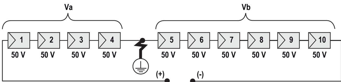
$V_a$  = voltage measured between + pole and  $\oplus$  = 200V
