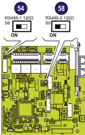
When connecting a single inverter to the monitoring system, activate the communication line resistance terminal by setting the switch 54 or 58 (to the ON position).
