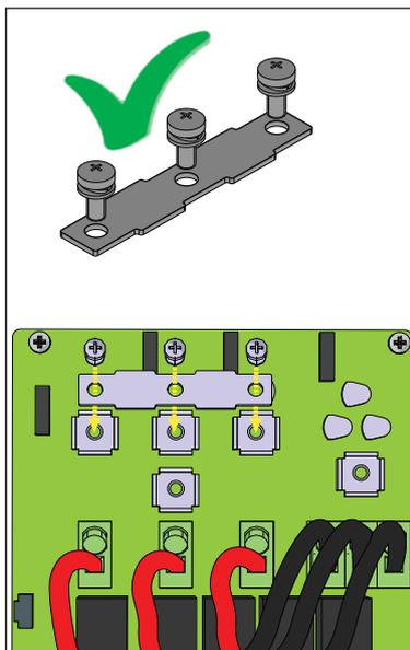
In the inverter -SX and -SX2 versions, the configuration of the input channels (MPPT) can be set in parallel. **Before carrying out this configuration, disconnect the strings from the inverter and open the AC disconnecter.** This means that the parallel bar (supplied) must be installed on the parallel MPPT connection points 41, and that the software setting “parallel channel mode” should be performed on the inverter; this setting can be done by different way:
