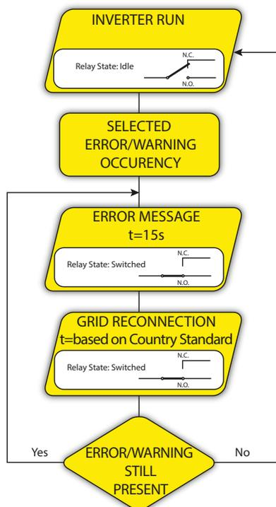
• **Alarm-Contact (alarm configurable - latch):**
