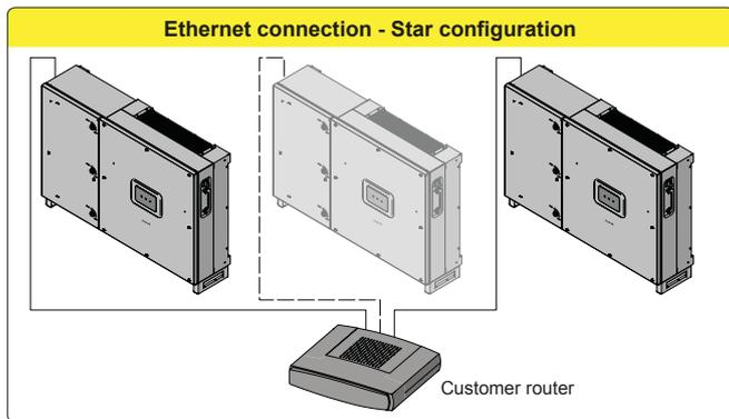
On each configuration of connection the maximum length of the cable must be 100m maximum between inverter – inverter and inverter – switch.
