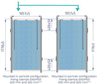
\*\*\*When a module is installed in portrait orientation on the pitched roof which has >45° slope, additional hook in the bottom of the module is required
