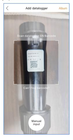
Note: Scan the datalogger SN, NOT the inverter SN.
