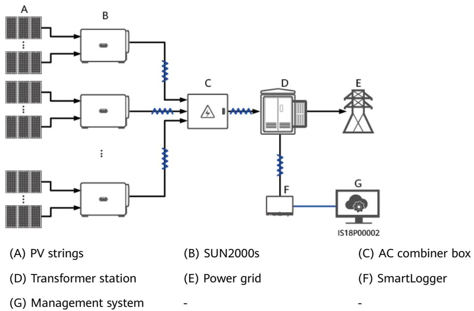
**Figure 2-3** MBUS networking application (double-winding transformer +SmartMBUS CCO)
