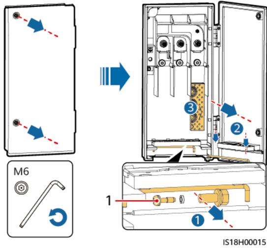
(1) Position for binding the ground screw
