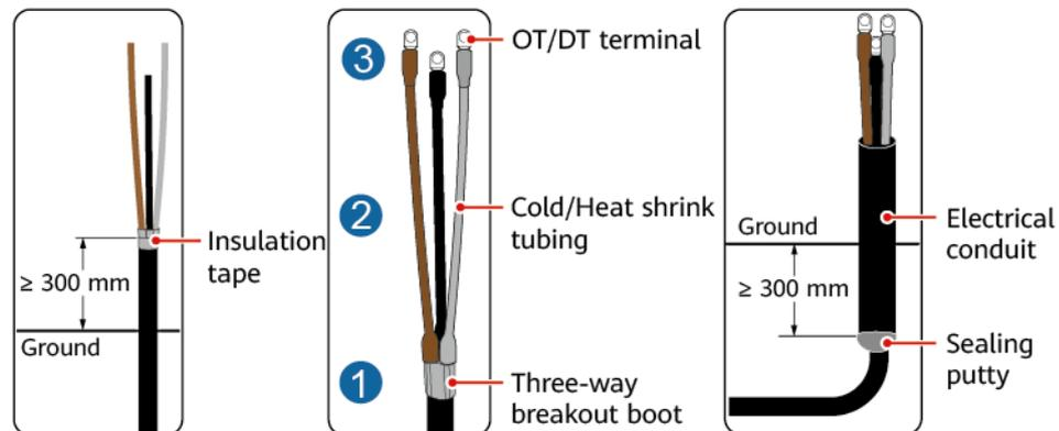
Figure 5-13 Installation completed
