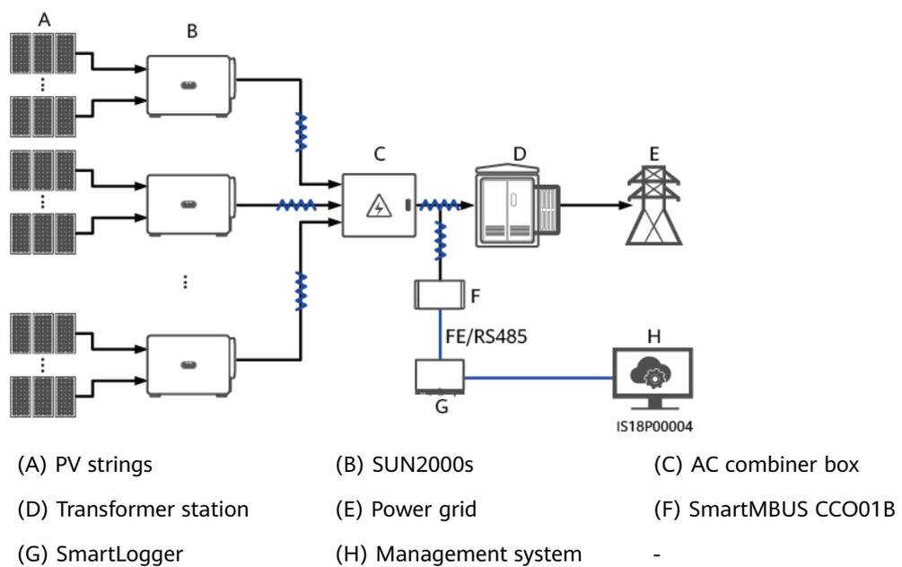
**Figure 2-4** MBUS networking application (double-split transformer+SmartMBUS CCO)
