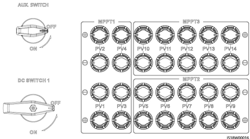
**Figure 5-15** DC terminals controlled by DC SWITCH 2
