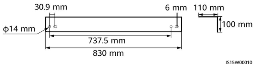
Preinstall the air baffle on the mounting bracket and then install the mounting bracket with the air baffle on the wall support.
