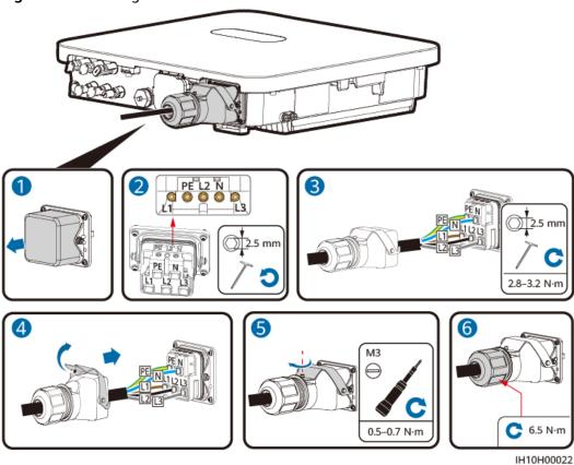
Figure 5-5 Securing the AC connector
