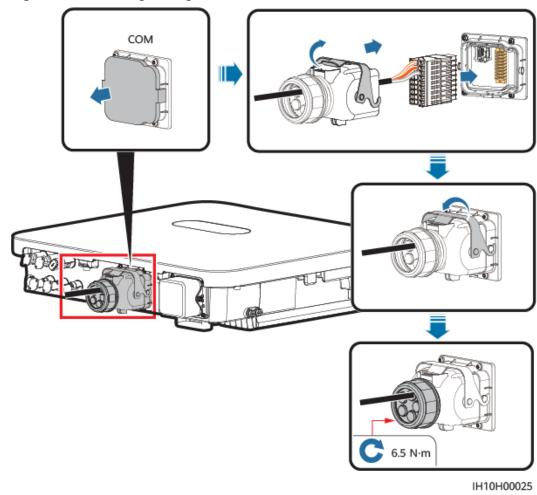
Figure 5-20 Securing the signal cable connector
