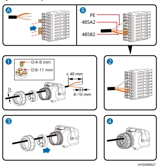
**Step 2** Connect the signal cable connector to the COM port.
