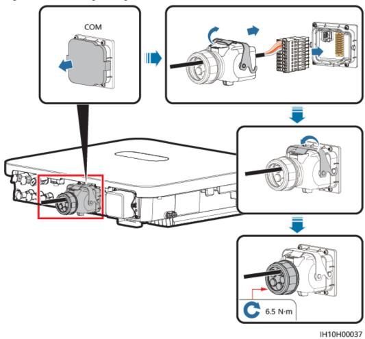
Figure 5-29 Securing the signal cable connector
