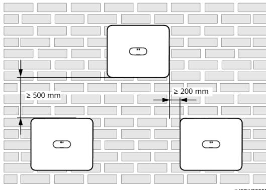
Figure 4-4 Triangle installation mode (recommended)
