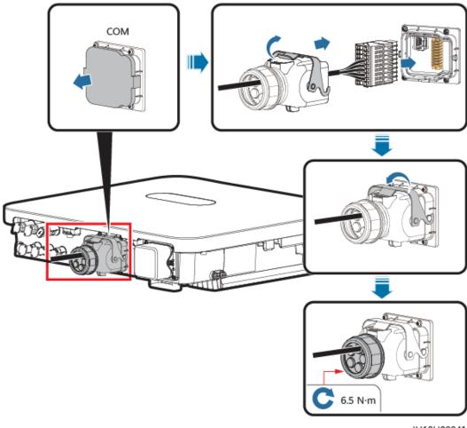
Figure 5-37 Securing the signal cable connector
