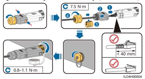
Figure 5-44 Installing anti-theft components for the Smart Dongle
