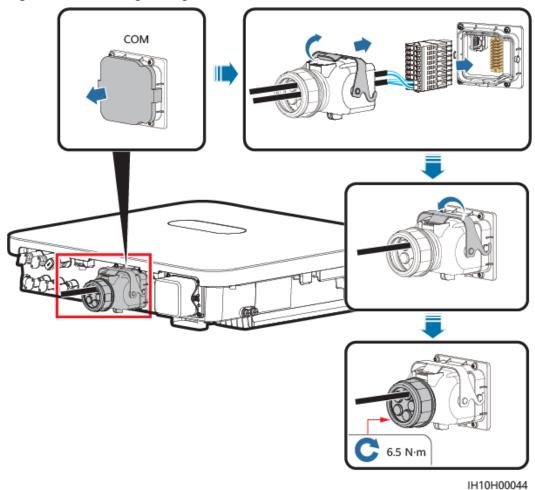
Figure 5-40 Securing the signal cable connector
