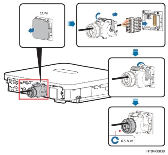
Figure 5-31 Securing the signal cable connector
