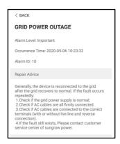
figure 7-8 Detailed Fault Alarm Information
