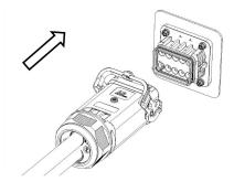
After the male and female insert the card point into the tracks lot, press the lock.
