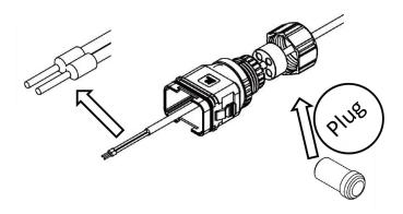
Insert the wires into the corresponding terminals.
