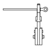
Use the crimping pliers to press the ground cable into the ground terminal, screw the ground screw with screwdriver as shown below:
