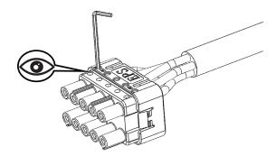
Insert the GRID end-core wire into the GRID end of the rubber core, observe the perspective hole cable in place, use S2.5 hex wrench to tighten the screws, torque 2.5±0.1N·m;
