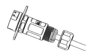
Tighten the connector's nut by the open-ended wrench with a torque 1.2±0.2N·m.
