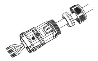
First, insert the EPS end cable into the EPS end of the rubber core. After the cable is in place through the perspective hole, tighten the screw using an S2.5 hexagon wrench with a torque of 2.5±0.1N·m.
