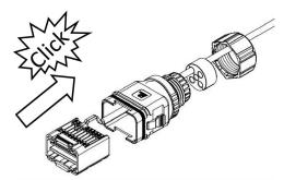
Install the plug into the main body and plug the holes without wires with a plug.
