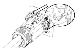
Tighten the screws with the S2.5 hexagon wrench with a torque of 2.5±0.1Nm. Installation completed.
