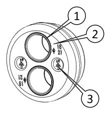
Note: If the outer diameter of the cable is greater than 18mm, remove part 1. When 4-core wire is used, Ø6 holes are ground wire through holes. Remove part 3.
