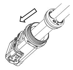
Tighten the nut with an open-ended wrench. (torque 10.0±0.1N·m, Complete the installation)
