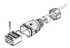
Arrange the core line, the rubber core area must not appear to ride the line. The rubber core is loaded into the main body and accompanied by a"click" sound.
