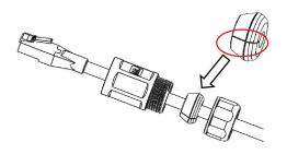
Stuck into the network cable through the gap on the sealing side.
