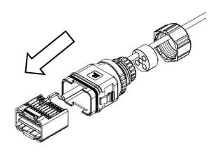
And use a screwdriver to crimp the wire, screwing torque 1.2+/-0.1N·m.
