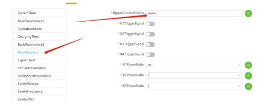
Firstly make sure that the ripplecontrolEnable switch is in the Enable state, which indicaties that the ripple control function has been turned on. The following K1-K4 Triggersignals function to display the status of ripple control, and K1-K3 power ratio indicates the corresponding power ratio.
