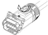
Align the female end with the male end in the anti-stay position.
