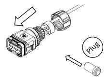
Lock wire nut screwed onto the body, torque 2.5+/-0.1N-m, then complete installation.
