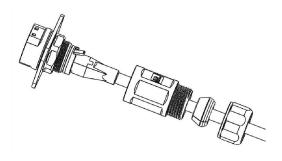
Tighten the connector mainbody by the open-ended wrench into the RJ45 panel mount connector with a torque 1.2±0.2N·m.
