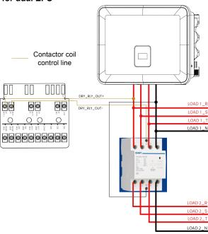
Load1 is directly connected to the EPS port and only loses power when the EPS stops outputting. Load2 is connected after the contactor and will shut off once the SOC drops below a certain level, causing the contactor to disconnect.
