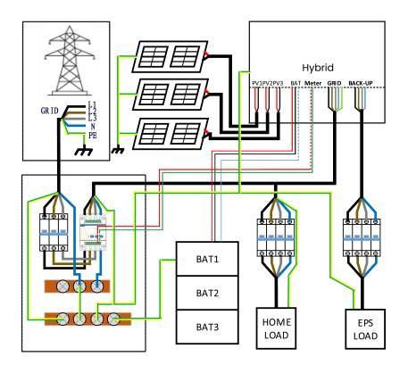
This diagram is an example for an application in which neutral is separated from the PE in the distribution box.
