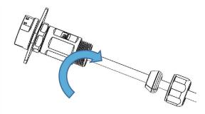
Insert the sealing plug into the main body of RJ45 cable end connector.
