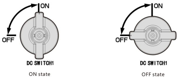
Fig 9.8 DC switch status
