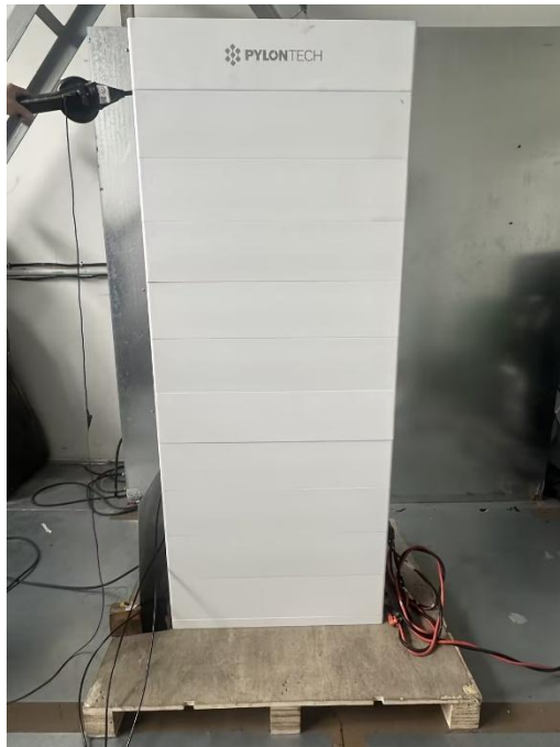
Photograph 4: Set-up for immunity test of electrostatic discharge
