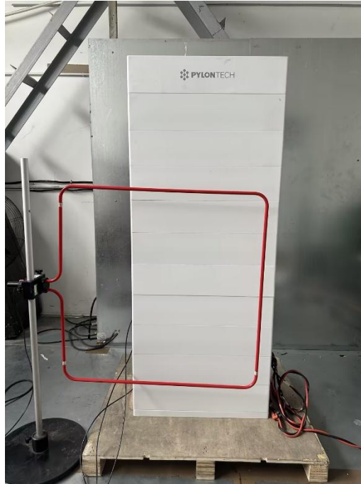
Photograph 5: Set-up for immunity test of power-frequency magnetic field
