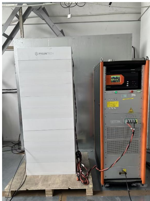
Photograph 6: Set-up for immunity test of surges
